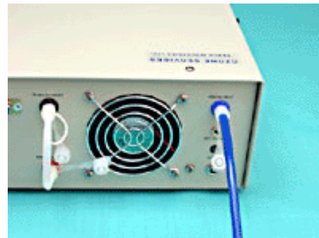
Attaching tubing to generator
