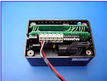
Upgrade port connected to terminal. • Black --> #4 Terminal • Gray --> #5 Terminal • Red --> #6 Terminal
