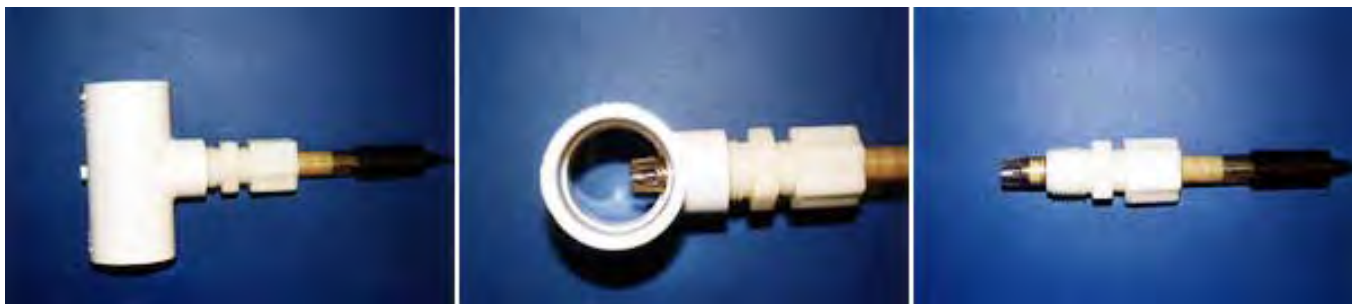
Slim ORP (or pH) Probe installed in a pipe
