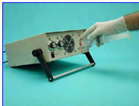
Continue holding down toggle switch while filling. When the syringe is full, the release of the down-pressure on the toggle switch turns the syringe port OFF
