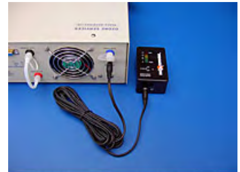
C30Z Ozone Monitor linked with Ozone Instrument EXT port.
