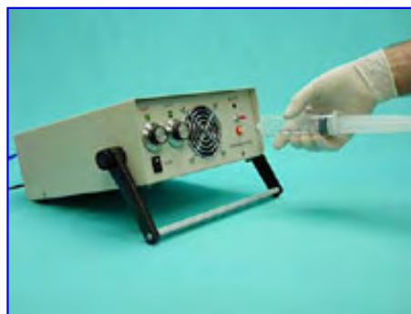
Continue holding down toggle switch while filling. When the syringe is full, the release of the down-pressure on the toggle switch turns the syringe port OFF
