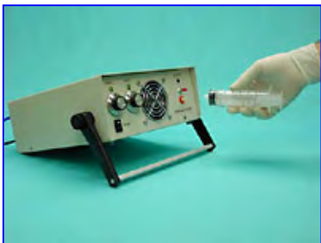
To fill a syringe, move it to the syringe port
